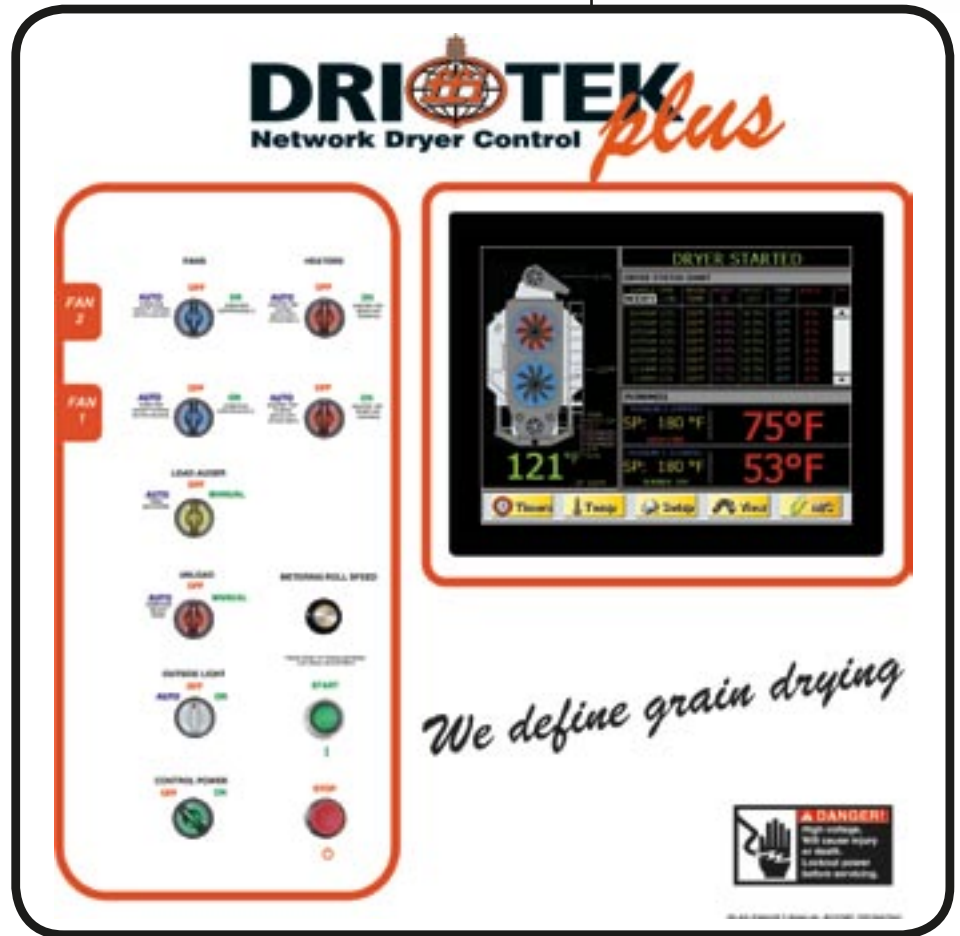
Computerized DRI-TEK Plus Control Panel Layout with Touch Screen Monitor
